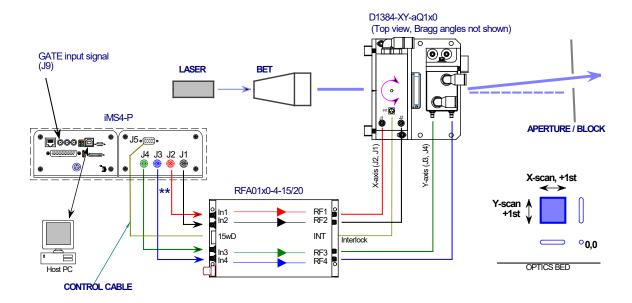
Note change in RF connections between IMS4 and RFA amplifier
